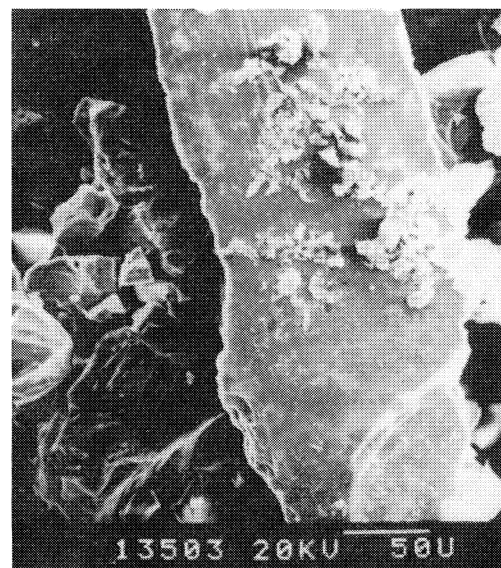
Fig. 1. SEM photograph of an Si particle coated with polypyrrole, Ag and Pt. Metallic deposits are seen as small white areas randomly distributed on the surface.
